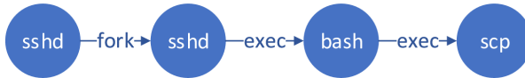
Fig. 2. The sshd daemon process forks a child process and the child process further spawns other process for various functionalities (secure copy).
